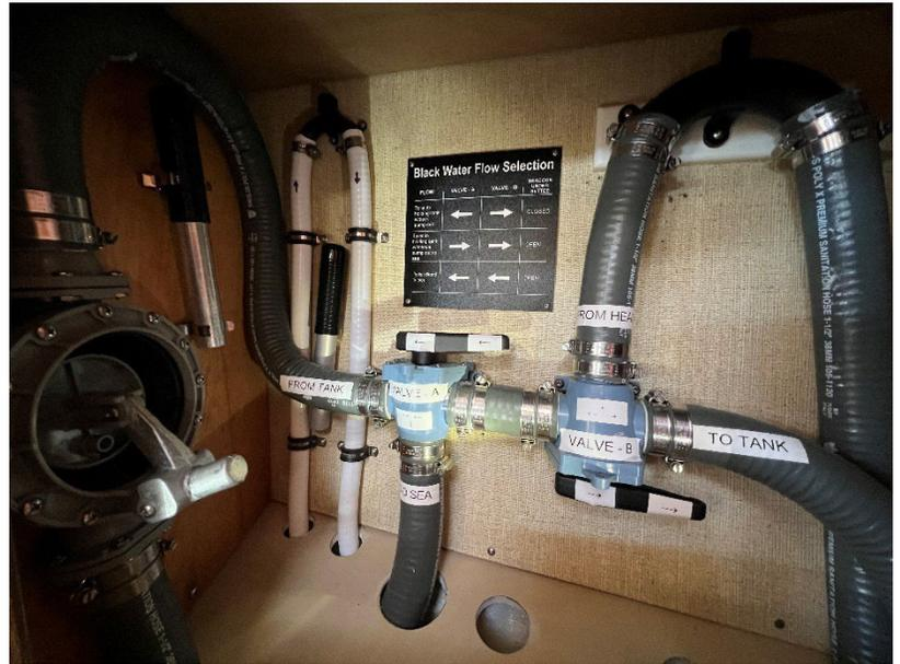
There are two Y-valves and one seacock that control the flow of waste from the toilet or tank. The Y-valves and manual overboard discharge pump are located in the salon, behind the port settee seat back (see photo above). The configurations are as follows (refer to the Flow Selection placard and valve photos - see photos on right and below). The arrows on the placard indicate which direction that the arrows on the valve handle should point.
