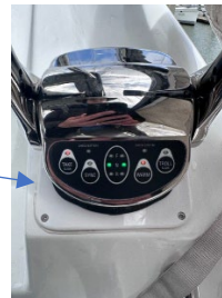
Figure 2. Starting Position: Neutral, “Take Slow” and “Warm” (both buttons are orange)
