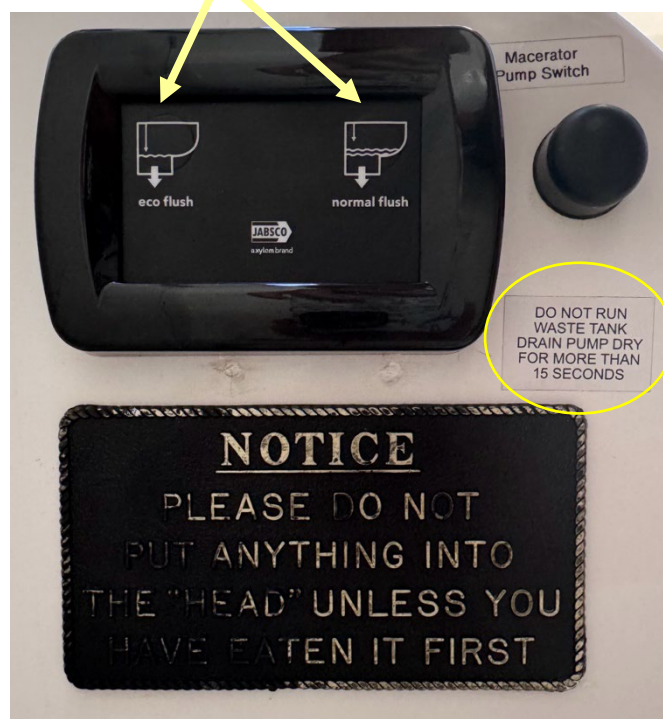
Eco/normal flush = less/more water
