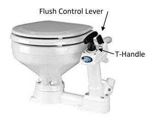
bring water in and out, then back to Shut ( ) to empty the bowl. If it gets hard to flush, try "oil and vinegar". SJS staff puts vinegar and vegetable oil in the head cabinet. Vinegar sanitizes and reduces odors. A tablespoon of vegetable oil flushed will lubricate the valves and seals, making pumping much easier as well as more efficient.
