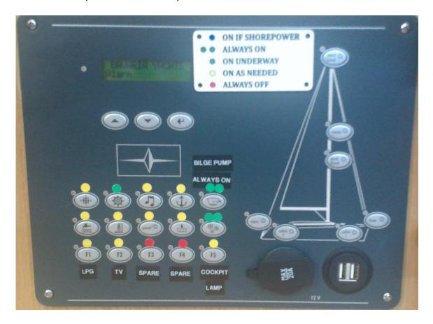
The top left section of the panel is an LCD display and controls. You can page through monitors of forward and aft fresh water tanks, holding tank, starter battery,
