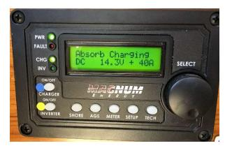
is the normal state of the charger / inverter and is left in this state. Any time AC power is connected to the ship, the charger will evaluate the quality of the power and once satisfied it is appropriate, it will start charging all batteries.
