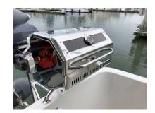
yellow manual gas valve must be opened for the BBQ to receive propane. Be sure to close the yellow valve and shut off the propane solenoid when done.
