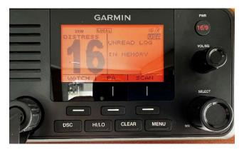
• Newer VHF radios such as the one on this vessel have several channel numbers that are now four digits, not two digits. This reflects a new standard. All affected channels will be in a format of 10xx, for example, channel 80A is now channel 1080. You can still operate the same as before, just the naming has changed for this new standard. Refer to the new listing in the Charter Guest Reference Manual binder on board, section 7, VHF Procedures & Weather Reporting.
