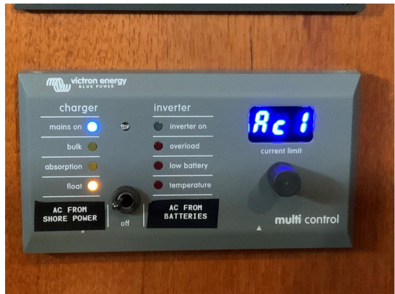
Inverter selected for shore power charging
