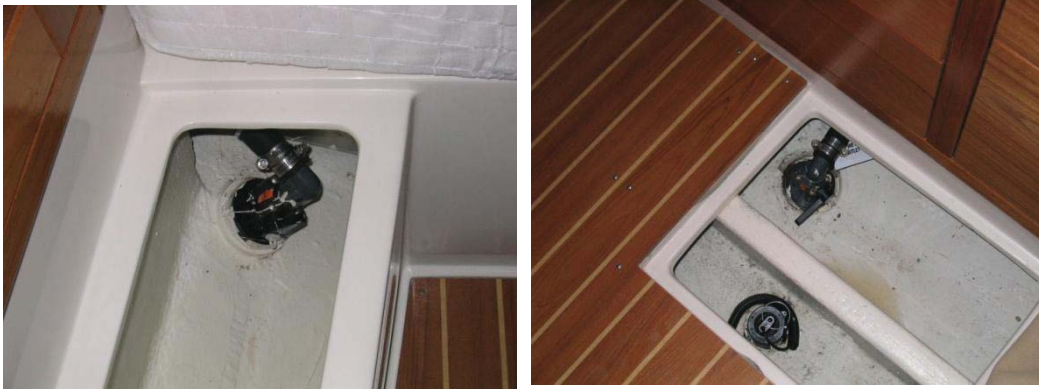
Aft Head Macerator Thru Hull (Starboard aft cabin seat) Fwd Head Macerator Thru Hull (Forward cabin sole)
