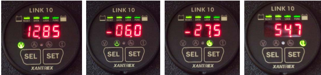
voltage amp draw *amp hours drawn down 27.5 54.7 hrs left at current draw *Note: beyond “-200” causes damage to batteries
