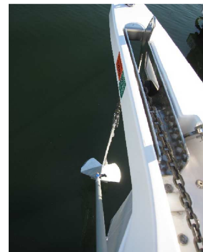
"SNUBBER" READY – hook on chain outside of roller, keep tension on lowering
