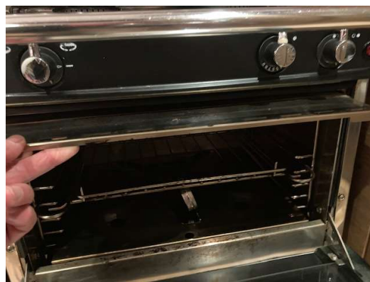
Figure 1. Heat shield pulled out at top of oven protects plastic knobs above when using the broiler.
