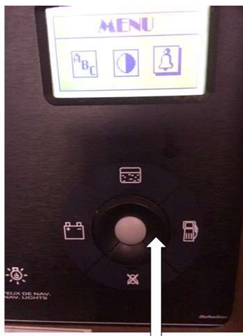
Press right button twice to move cursor to Alarm MENU then press center button to select
