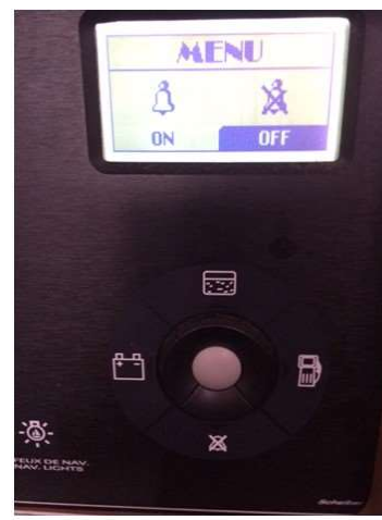
Press right button to move cursor to OFF then press center button to select
