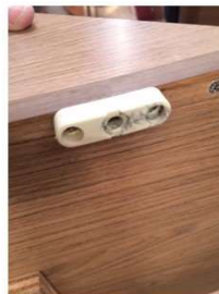
...should rest in the hole in the middle of the white flange on the bottom of the drawer
