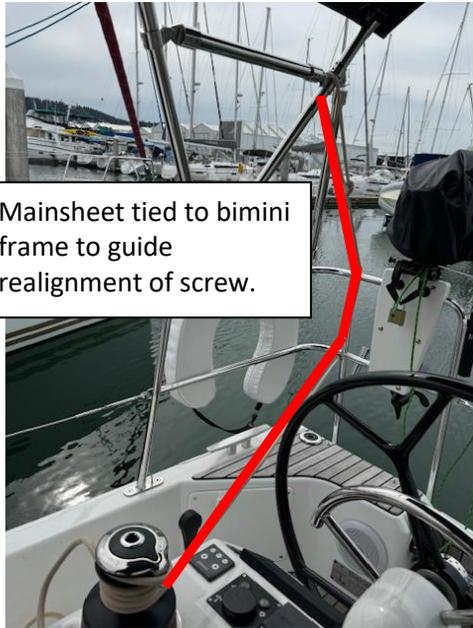
Mainsheet tied to bimini frame to guide realignment of screw.
