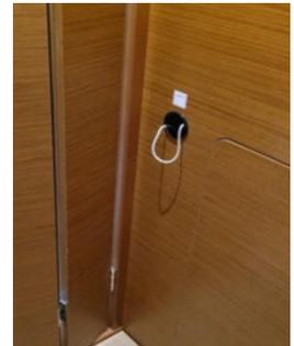
Help to prevent fires by turning the propane solenoid switch off when not using the stove or BBQ while not in use. Refrain from having open flames below, in the cockpit and on deck.
