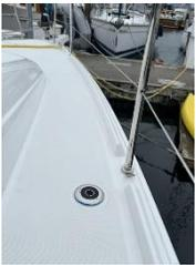
The deck fitting for the water tank is on the starboard side next to the third stanchion from the bow. The fitting is marked “Fresh Water” and has a blue ring between the fitting and the deck.
