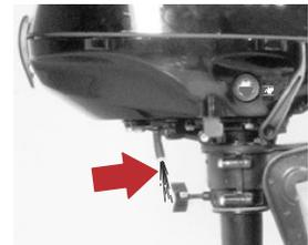
Pull the starter rope slowly until you feel the starter engage, then pull rapidly to crank the engine. Allow the rope to return slowly. Repeat until the engine starts.
