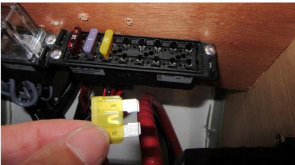
A fuse protects an electrical circuit from excess current. If it blows, you must replace it with another fuse of the same rating.
