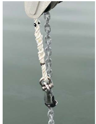
Chain hook attached-this should be let out 20-30’
