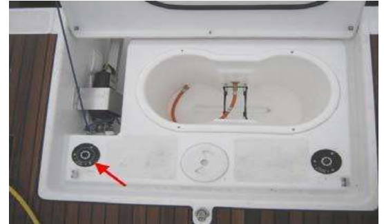
Aft water tank fill port (red arrow).
