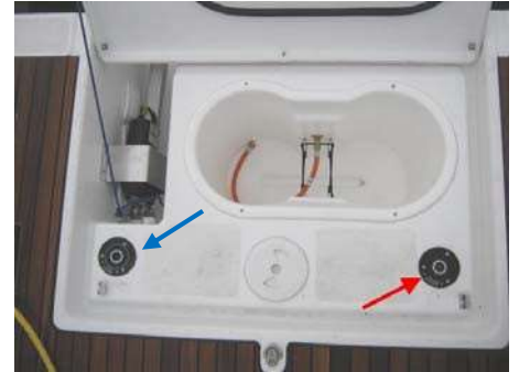
Fuel tank fill port in propane locker (red arrow); aft water tank fill port (blue arrow).
