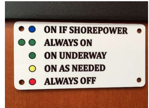
Default electrical panel switch settings.
