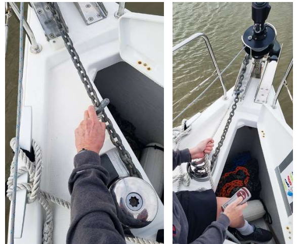
Attaching the snubber line to the chain (left) and keeping tension on the line while it is being deployed (right).
