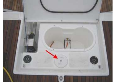
Propane locker with emergency tiller access (arrow), diesel fuel port (right) and aft water tank port (left).
