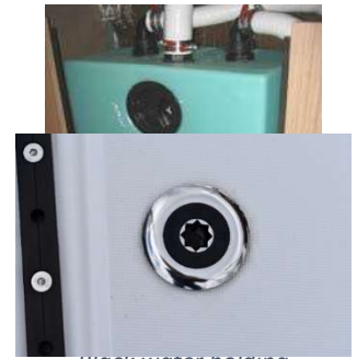
Black water holding Waste tank pump-out access ports located on starboard deck above holding tanks.
