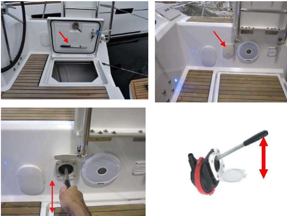
Operating the manual bilge pump (handle clipped under starboard cockpit transom locker hatch).
