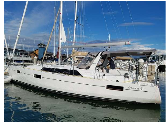
Furled mainsail & headsail - note mainsail clew exposed and one wrap of jib sheets around genoa.
