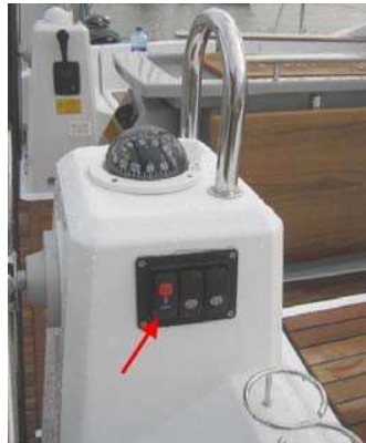
Swim platform controls (red arrow) – the other switches control cockpit lighting.
