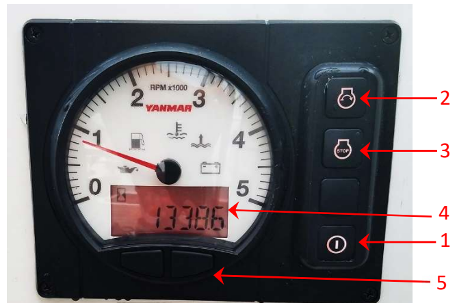
Engine controls: (1) Power ON/OFF, (2) START, (3) STOP, (4) Engine data, e.g., hours, (5) Toggle LCD engine data display.
