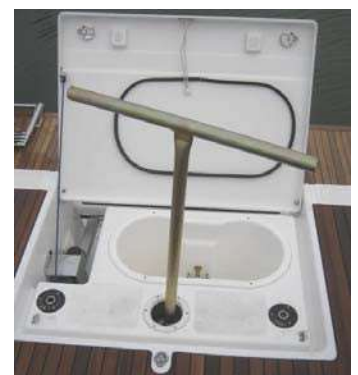
Emergency tiller installed.
