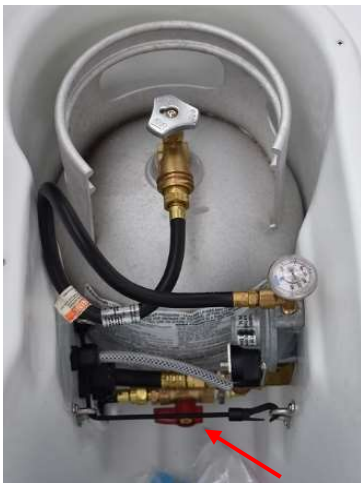
Propane tank with master valve (top) and red BBQ valve (red arrow – valve in open position).
