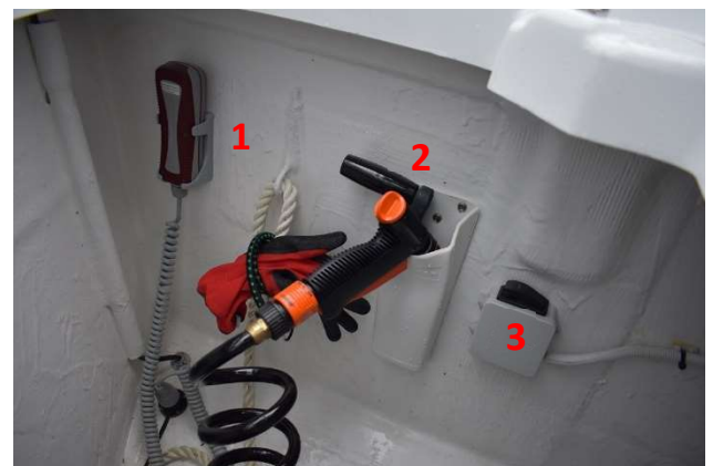
Anchor locker with windlass controller (1), wash-down hose (2) and wash-down pump switch (3).
