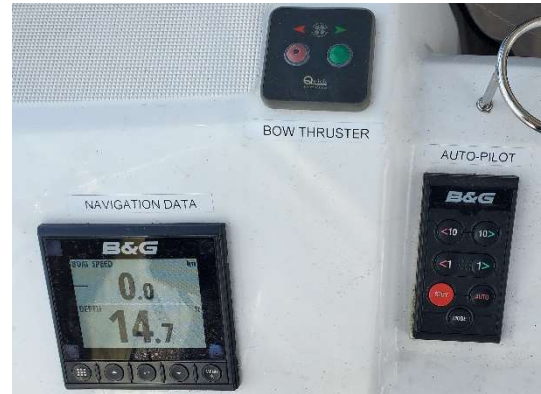
Triton 2 navigation data, auto-pilot and bow thruster controls.
