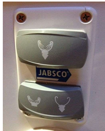
Forward head rocker switches.
