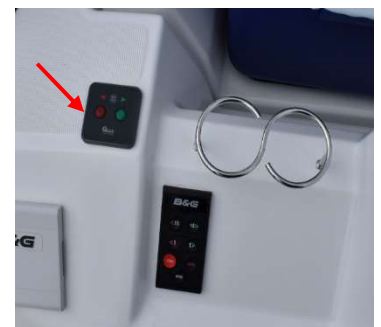
Bow thruster controls (red arrow).
